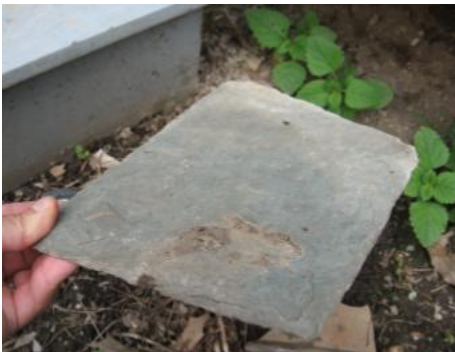
Detail image [LEFT] shows failed slate tile found at grade, west elevation of Hanley House. This was likely used to patch a failed cement tile during the past thirty or so years. It should be noted that slate tiles are significantly heavier than cedar shakes and cement tiles, and so should not be used to patch large areas of the Hanley House roof without a more thorough understanding of existing roof framing design and load capacity.
