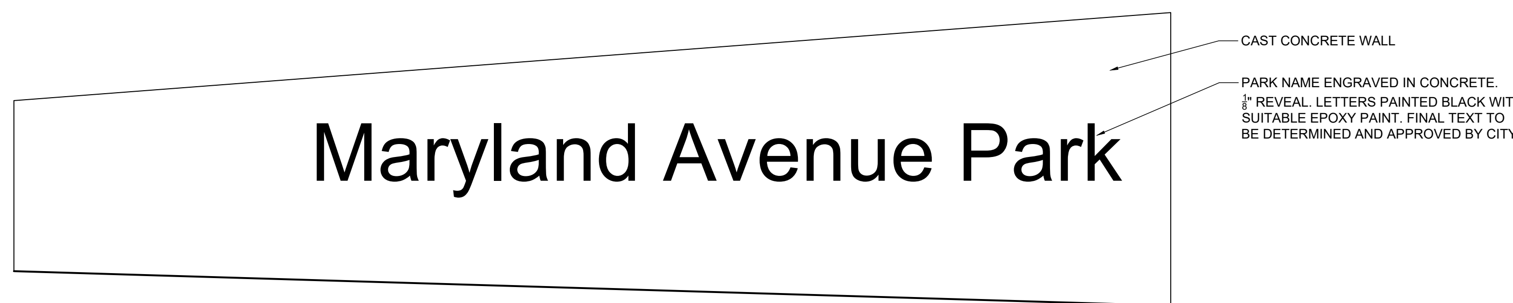
A ENTRY SIGN WALL ELEVATION SCALE: 1"=1'
